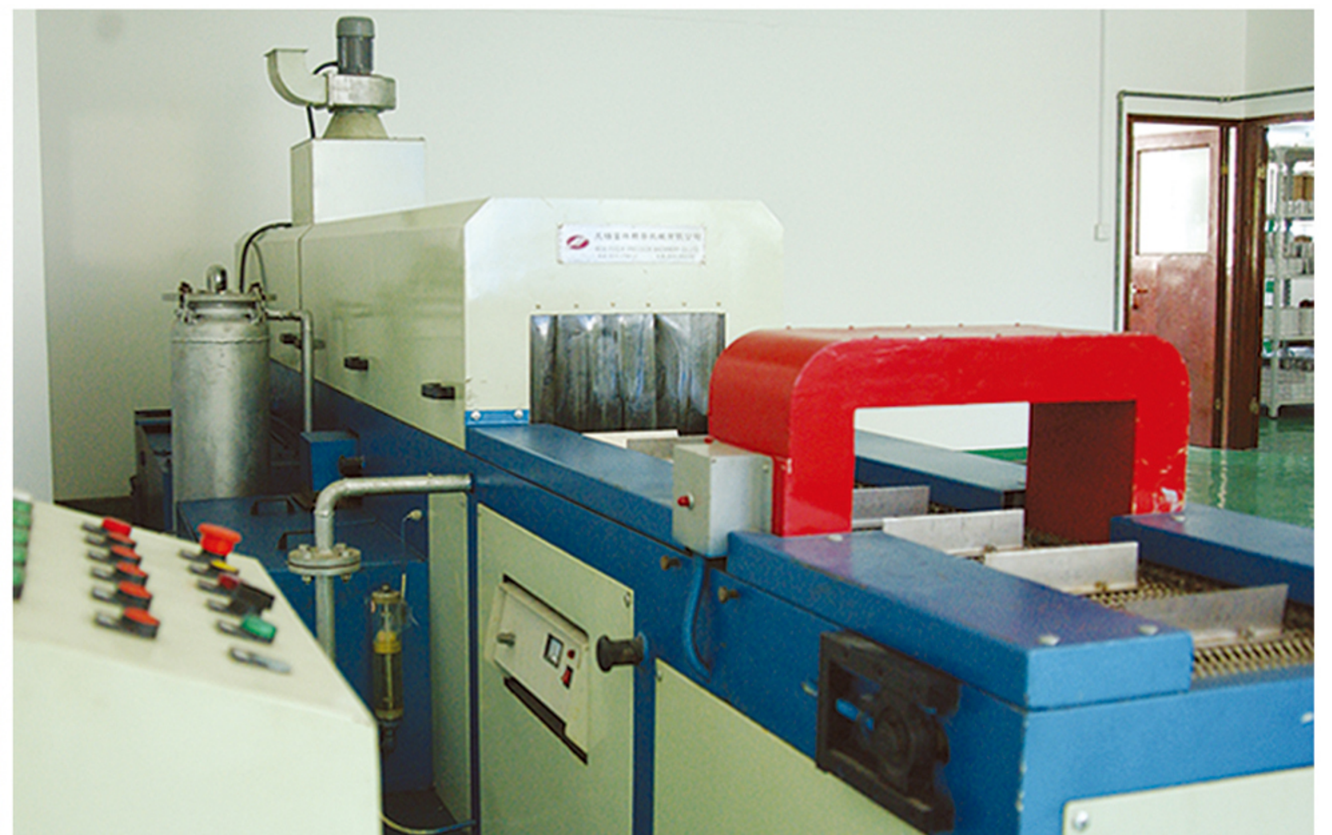
Ultrasonic Clean Line
